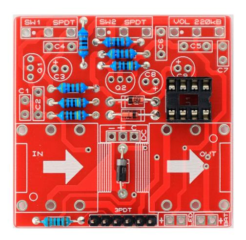
First of all place the IC sockets (without the ICs). Pay attention to the orientation! The small notch in the socket should be oriented as indicated in the PCB.
